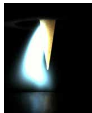
Low-quality tungsten: typically sideways arc ignition, the arc flashes and wanders slowly to the electrode tip which has to be cut off and reground.
