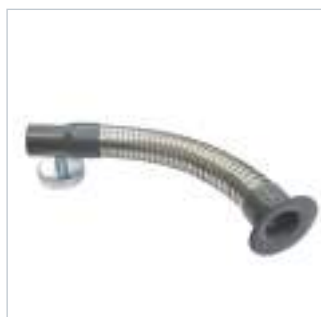
MOUTH PIECE ROUND Ø50 MM Conic extraction mouthpiece with steel hose and magnet for mounting on 51 mm flex hose.
